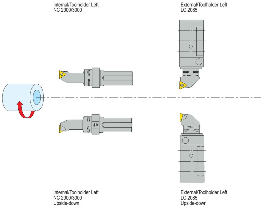
2000 = cylindrical type with drawbar, 3000 = cylindrical type with screw, 2085 = shank type.
