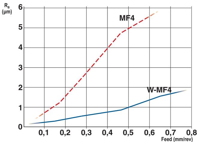
When applying a Seco High Feed W-MF4 wiper insert in stainless steel the diagram shows the superior surface finish achieved compared to a conventional insert in stainless steel. CNMG120408W-MF4 TM2501,  $a_p = 1$  mm, cutting speed tool life adjusted for feed in SMG M2 (stainless steel).
