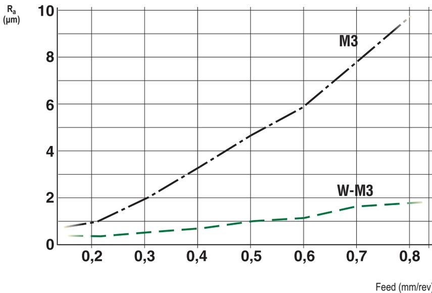
The outcome from using a High Feed Wiper insert can actually even eliminate the need for a separate finishing cut, which is indicated and described below.
