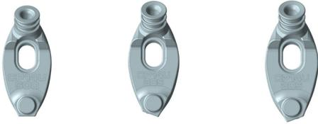
The coolant clamp executes many functions. It provides a secure and fast clamping of the insert by virtue of the spring loaded design with a single screw. It directs and orients the high pressure coolant jets straight and close to the cutting edge. The manufacturing flexibility of the coolant clamp allows it to have an optimised coolant channel with different hole diameters.
