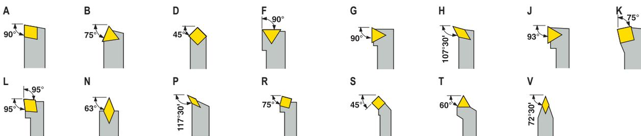
Now as seen earlier there are several demands and requirements on the generation of surfaces in turning. The above sketches on the codes for tool types give hint on the options connected to the position "3" in the below code key for toolholders.
