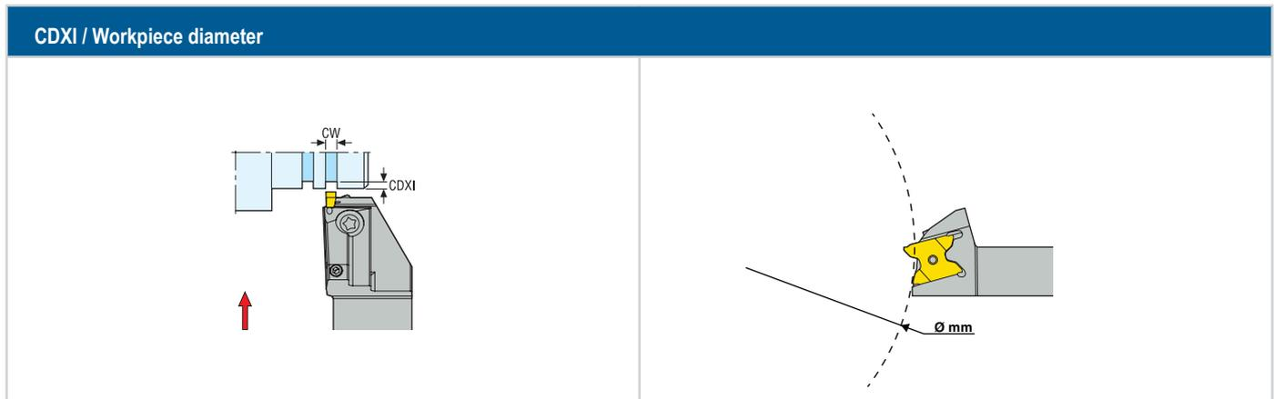
Maximum cutting depth CDXI is limited relative to workpiece diameter to avoid contact between workpiece and toolholder.
