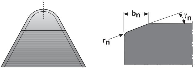
$b_n$  = Chamfer width
