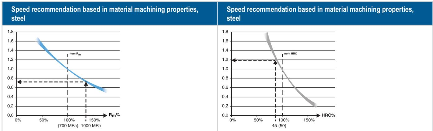
To further illustrate how the SMG P5 nominal v<sub>c</sub> can be adjusted to a more accurate recommended v<sub>c</sub> we need ultimate tensile strength R<sub>m</sub> data and in this case we use the EN 42 CrMo 4 quenched & tempered to R<sub>m</sub> = 1000 N/mm<sup>2</sup> according to above table (bold blue arrows).
