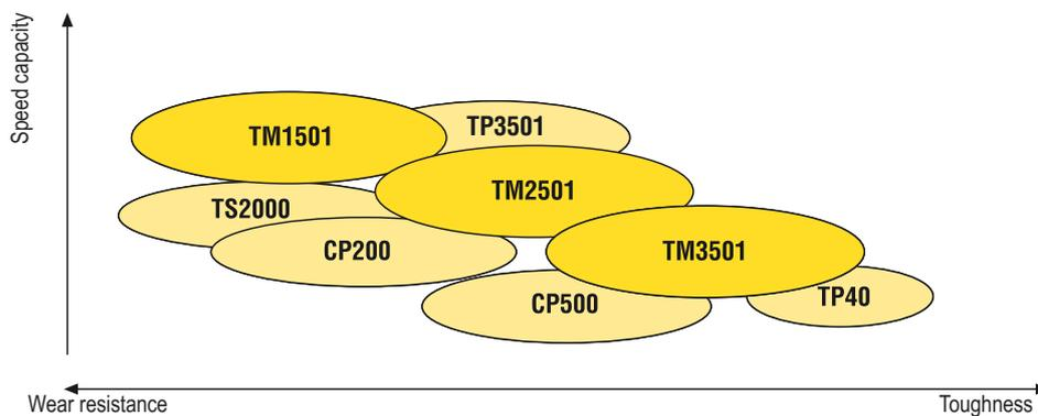
The well connected TM1501, TM2501 and TM3501 Duratomic grade chain covers applications in stainless steel turning, but also the thin PVD-coated TS2000, CP200 to CP500 complements the above high productivity CVD grades with reliability, but not at as high speeds as the Duratomic grades.
