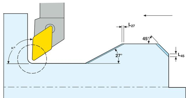
The High Feed geometry on a D-and T-style insert does not provide an exact corner radius.
