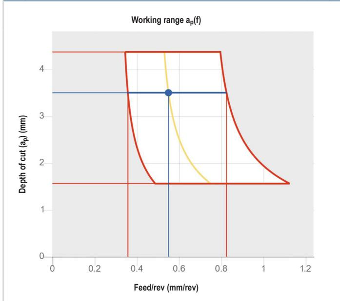
For a certain insert and chipbreaker combination there is a recommended working range and depend on several aspects in insert design and of machining conditions such as component and path.
