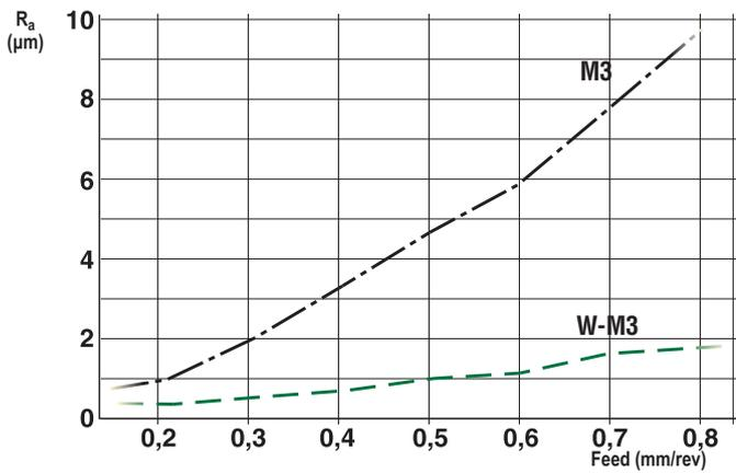
The diagram shows the superior surface finish in steel achieved with a Seco High Feed W-M3 wiper insert compared to a conventional insert. CNMG120408W-M3 TP2501,  $a_p = 1$  mm, cutting speed adjusted for feed, workpiece material: (steel) SMG P4. Note that opportunities to do the same surface finish comparison for each specific product and application when logged in on [www.secotools.com](http://www.secotools.com) under the Advanced Cutting Data section.
