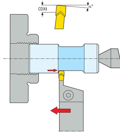
The deflection arising during turning causes a minor change of the actual tool length. This influences the received diameter on the workpiece.
