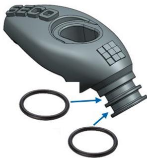
It is recommended that O-rings are checked regularly since the double O-rings are the coolant entry-point of the coolant clamps. When the O-rings are exchanged it is recommended to also make it a habit to exchange the screw to ensure pro-active high pressure operational safety.
